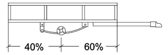
On a Tandem axle trailer The equalizer hanger is the point from which you will calculate the axle centerline measurements for tongue weight assessment.
